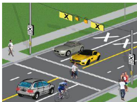
Figure 39: Typical signalized crosswalk design
